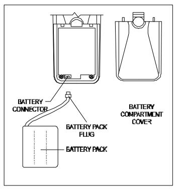
Remove the handset battery compartment cover by pressing the circular on the top side of the cover then silde it down.
